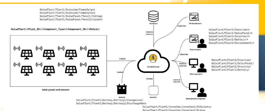
Caption: Data flow architecture of a remote monitoring system for a solar power plant
